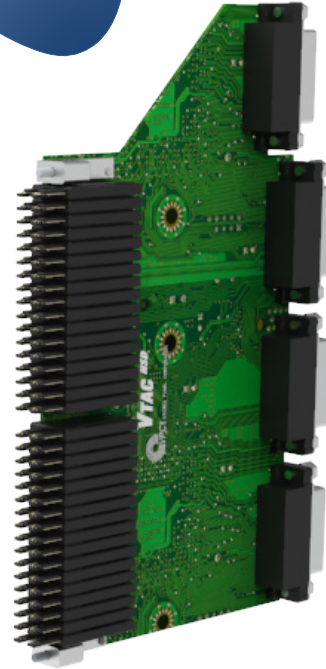
VTAC Right Angle Inserts Mounted to PCB
