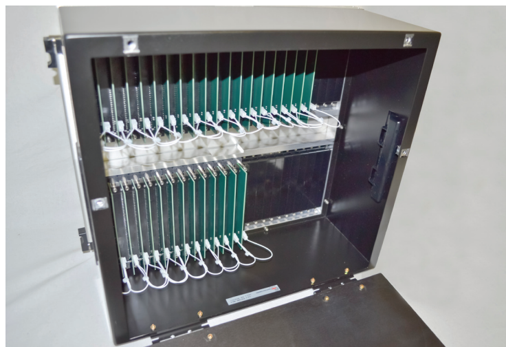
A 50 Module ITA Enclosure Slotted with PCBs
