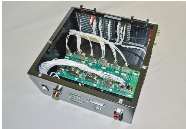
Enclosure with Secondary Connectors and Silkscreen Labels
