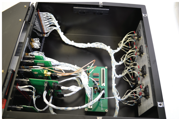
ITA Enclosure with Small PCB Wired to Another PCB
