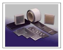
HiTherm materials are manufactured from natural graphite and a polymer additive. The addition of this polymer additive to highly conductive natural graphite minimizes the thermal resistance at low contact pressures.
