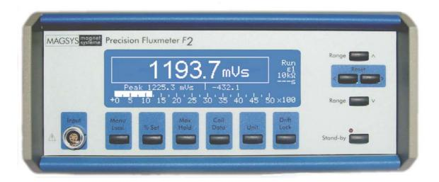
The Precision Fluxmeter F2 enables you to measure the magnetic values flux  $\Phi$ , flux density B, field strength H and polarization J. A coil made for your specific purpose is connected to the fluxmeter as a probe.
